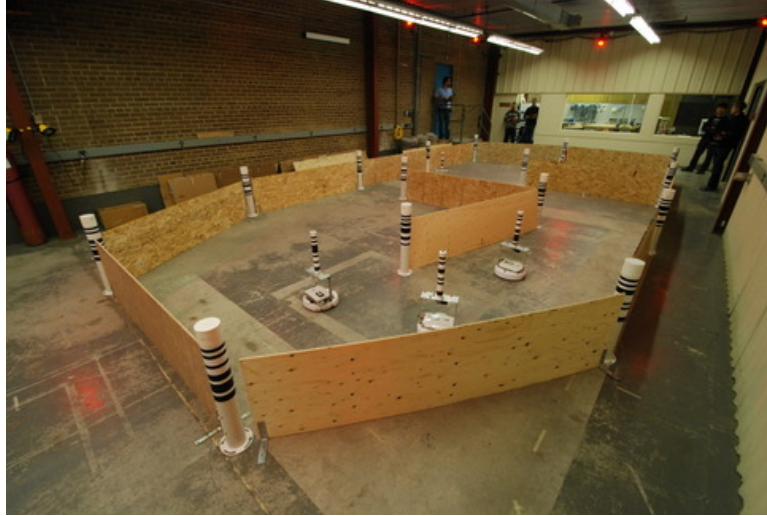
Figure 3.11: In sub-dataset 9, data collection was performed with barriers in the workspace to increase occlusions for measurements.
