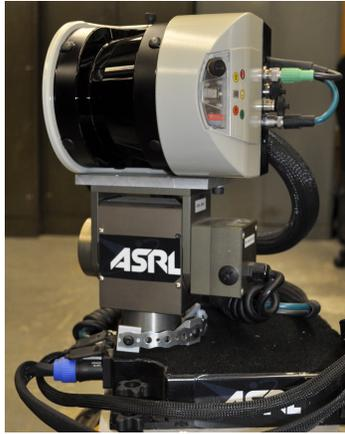
(a) A vertically scanning panning laser rangefinder composed of a laser mounted on a panning unit.
