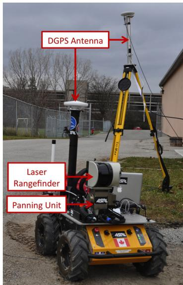
(a) The Clearpath Husky A200 rover used to gather the dataset. The relevant payloads are the laser rangefinder mounted on a panning unit, and the DGPS antennas for ground truth data.
