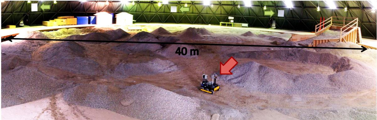
(a) A panoramic image of the UTIAS indoor rover test facility, with the rover used to gather the data identified by the red arrow. The terrain consists of gravel spread in a 40m diameter circular workspace, emulating scaled planetary hills and ridges. The reflective signs used for ground truth are highlighted by the green arrows.
