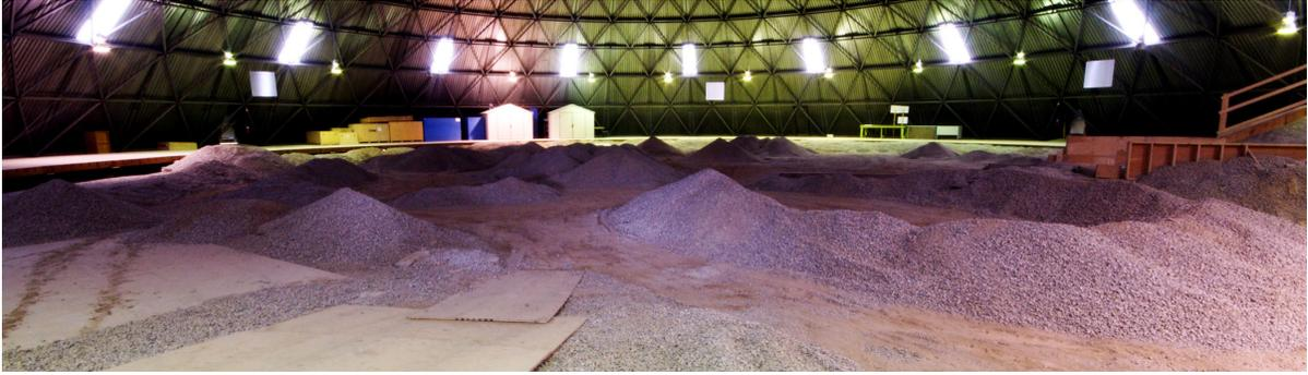
Figure 6.11: An image of the UTIAS indoor rover test facility. The terrain consists of gravel spread in a 40m diameter circular workspace, emulating scaled planetary features.
