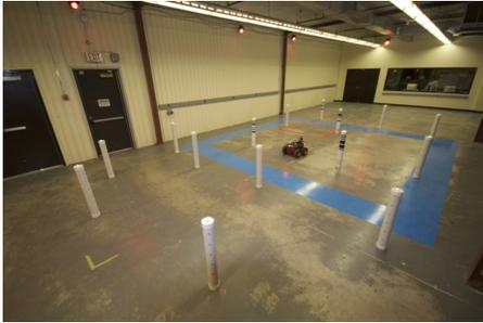
(a) The hardware consisted of a P3-AT mobile robot, a Hokuyo URG-04LX-UG01 laser rangefinder, plastic tubes, and a Vicon motion tracking system.
