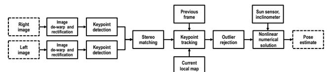
Fig. 2. Modified stereo visual odometry pipeline used in *network of reusable paths*. When repeating a route, we match the current image to the previous image to compute motion, but also to a local map of features stored relative to the path; this allows the robot to compute where it is relative to the path and steer back onto it.
