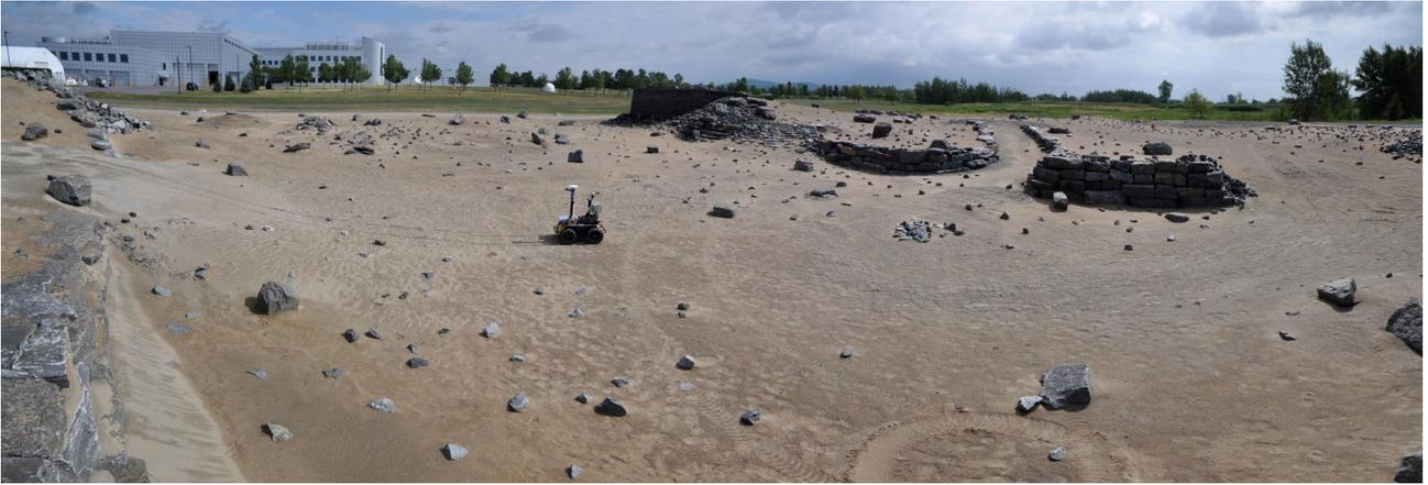
Figure 2: Rover traversing Mars Emulation Terrain (MET). The rover uses stereo vision for navigation and obstacle avoidance, and a 3D laser rangefinder for mapping and localization.
