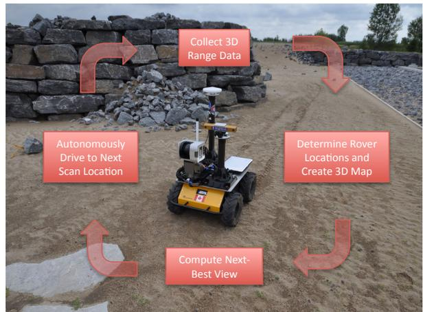
Figure 1: Operational cycle for 3D site mapping. The rover collects 3D range data while stopped. A batch SLAM algorithm computes the rover pose and creates a consistent 3D map. The operator selects the next-best view (NBV) based on three computed metrics. The rover autonomously drives to the NBV and the cycle repeats.
