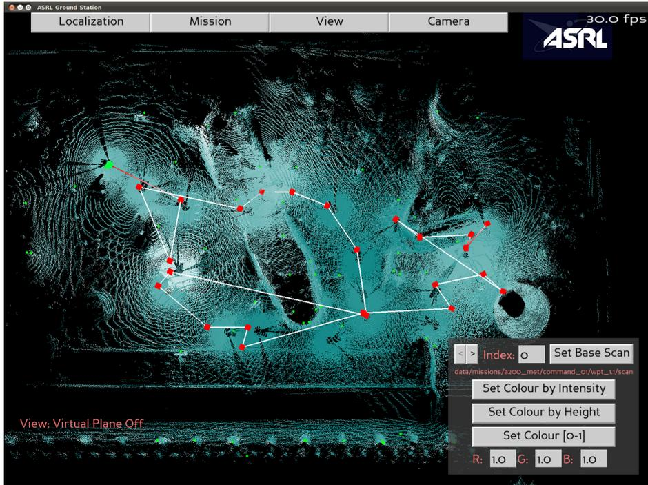
Figure 9: Ground Station software illustrating the map after the 25-scan traverse. The terrain is shown as a 3D point cloud, and overlaid are the scan locations (large green and red boxes) with lines between them indicating the order. The green box is the starting location of the mission. The small green circles on the map are landmarks.
