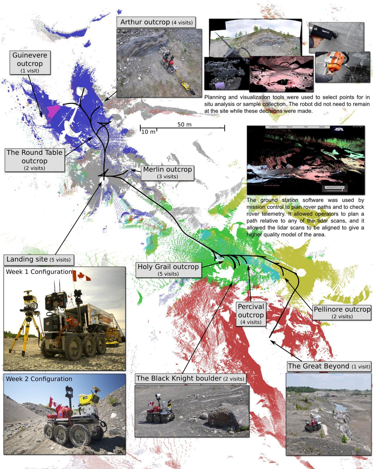
Figure 8. An overview of the network of reusable paths (the black line) at the end of the mission. NRP allowed the robot to return to any position that was previously visited. This meant that mission control could delay analysis or sampling decisions at one site, and still continue to carry out operations at other sites. At the end of week two, the total length of the network of reusable paths was 440 m, and by then the robot had driven a total of 3 920 m.
