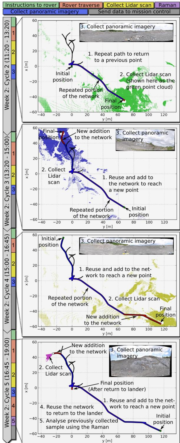
Figure 10. Parallel exploration was done between the odd and the even command cycles. In cycle 2 of week two, the robot collected a lidar scan and panoramic imagery. In cycle 3 the robot was sent to another area to collect more data while mission control reviewed the data from cycle 2. In cycle 4 the robot reused the network to return to the end point of cycle 2 and continue exploring while the data from cycle 3 were reviewed.
