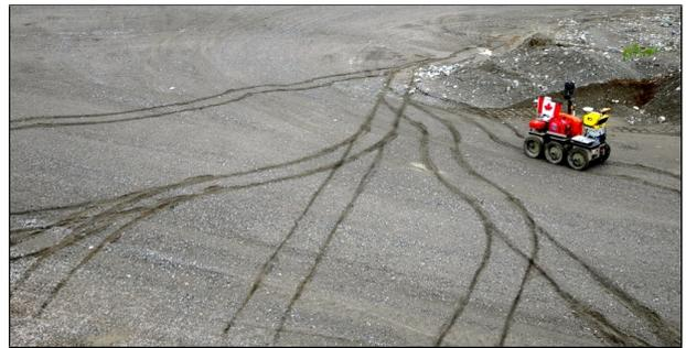
Figure 1. A robot operating on a network of reusable paths. The robot is repeating a previously driven path (in its own tracks) to return to a previously visited position.
