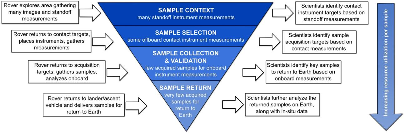
Figure 5. A methodical down-selection process is enabled by a network of reusable paths. There are a decreasing number of samples at lower levels to accommodate the higher resource usage per sample.
