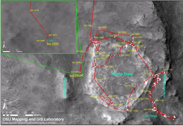
Figure 2. Traverse map at sol 2555 for the Mars Exploration Rover; Spirit. Credit: OSU Mapping and GIS Laboratory, NASA/JPL/Cornell/University of Arizona.
