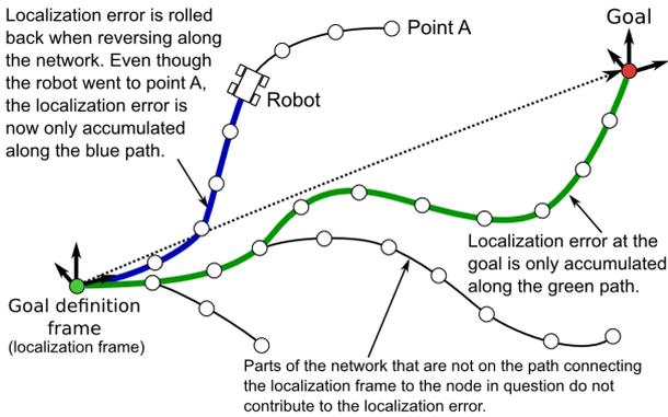
Figure 6. The localization error is only due to the errors in the transformations at the edges that connect the node used as the localization base frame, and the node against which the rover is localizing. This means the localization error at the goal is only accumulated on the final path to the goal from the goal definition node, and that error is rolled back when reversing along a previous route.
