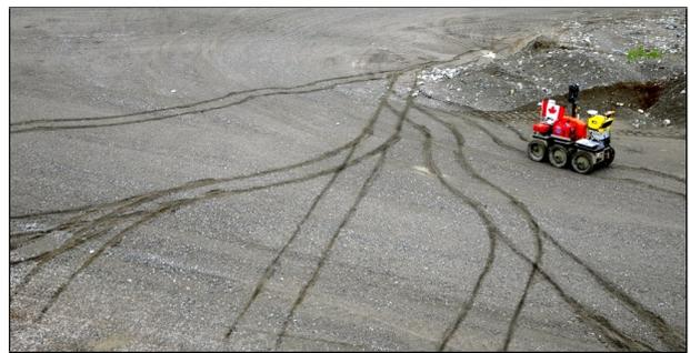
Figure 1. A robot operating on a network of reusable paths. The robot is repeating a previously driven path (in its own tracks) to return to a previously visited position.
