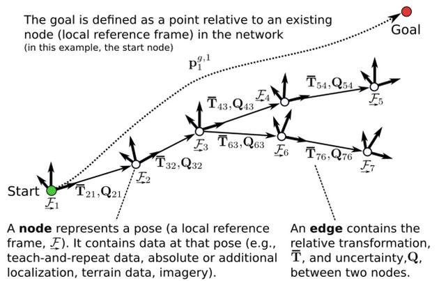
Figure 4. Definition of the key components of the graph structure used in a network of reusable paths. There is no privileged coordinate frame, everything is relative.
