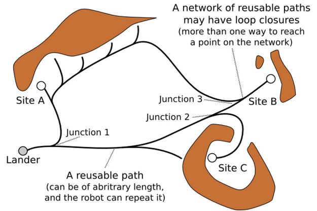
Figure 3. A simple network of reusable paths is shown in black. The robot can return to any point on the network and can grow the network into new areas. To go from site B to C, the rover reuses the previous paths by traveling through junction 3 and then 2, before going to site C.
