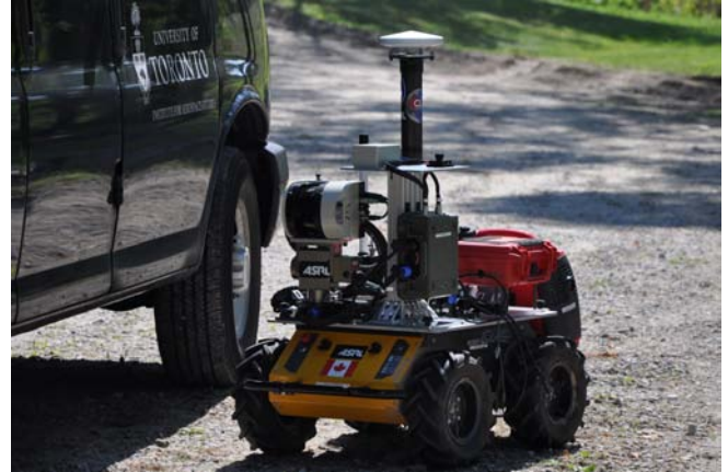
Figure 1. The ASRL Clearpath Husky A200 equipped with a laser rangefinder, star tracker, and inclinometer.
