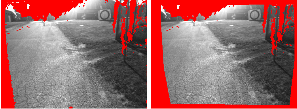
Figure 3.3: On the left we have an image that has been warped with the initial pose guess, \mathbf{T}_{\text{op}} . Invalid coordinates are shown using a red mask. The mask on the right is created by further perturbing the pose in individual DOF in a small area around \mathbf{T}_{\text{op}} . This gives us a buffer so the mask will stay the same while the pose updates during iterations.
