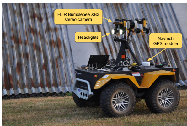
Figure 2.12: The Clearpath Grizzly robot with a forward-facing FLIR Bumblebee XB3 stereo camera, headlamps, and a Navtech GPS.
