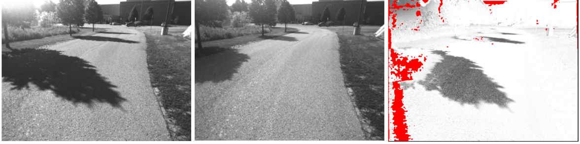
Figure 3.2: The live image (left), the map image (middle), and a weight image (right) displaying the weights computed by the Geman-McClure robust cost function. Dark pixels correspond to low weights. We see that areas with changing shadows are downweighted. Red pixels are excluded.
