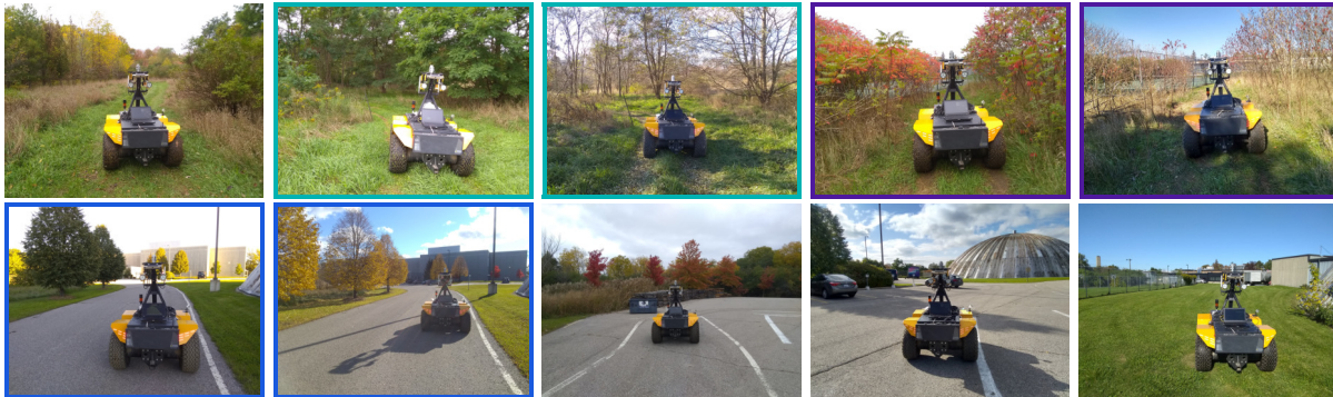
Figure 6.24: The robot repeating the path for the seasonal experiment under different appearance conditions. The coloured frames indicate pictures taken in the same location at different times.
