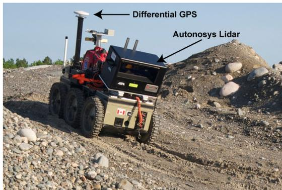
(a) The ROC6 mobile rover, equipped with an Autonosys LVC0702 lidar and a Thales DG-16 Differential GPS unit.
