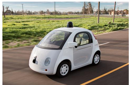
(b) A depiction of Google’s autonomous vehicle prototype in 2015. The driverless vehicle uses a combination of lasers, radars, and cameras to safely navigate roads shared with other civilian drivers. (Credit: Google)
