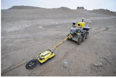
Figure 8: Rover driving in its own tracks during visual homing.
