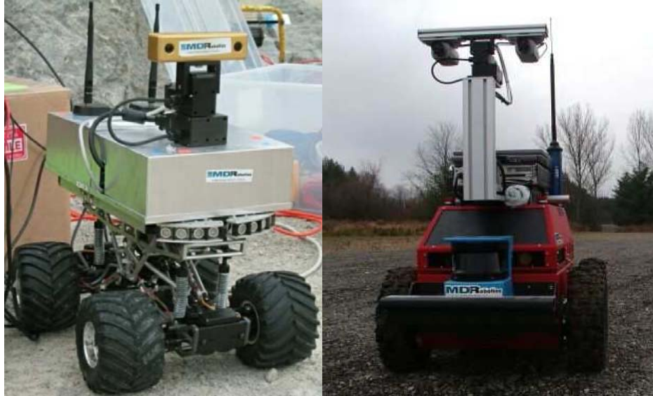
Figure 8: (left) Custom rover with Bumblebee stereo camera. (right) ATRV Jr rover with custom stereo camera.
