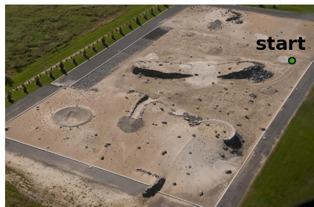
Figure 10. : The Mars Emulation Terrain at the Canadian Space Agency in Montréal, Canada. The artificial terrain spans 120×60 metres and contains many structures that introduce elevation changes. Scientifically significant rocks were hidden throughout the terrain for the sample-return analogue mission. Start location of the analogue mission marked with a green dot.
