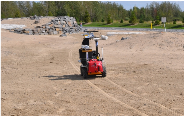
Figure 2 : A Husky rover revisiting a point on a network of reusable paths. The NRP algorithm is accurate enough to enable the rover to repeat along the path in its own tracks using only a stereo camera.
