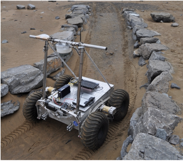
Figure 13. : The Juno rover being teleoperated to ‘Cardasia’ under a communications delay. The path to the site leaves very little clearance on either side of the rover, but the side-mounted cameras (with distance overlays) allowed the rover to be driven safely through the hallway.
