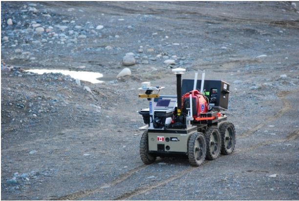
Figure 4 : The RobuROC6 robot using NRP to autonomously repeating a traverse during a Sudbury lunar-sample-return analogue mission. The algorithm is accurate enough for the rover to drive in its own tracks.
