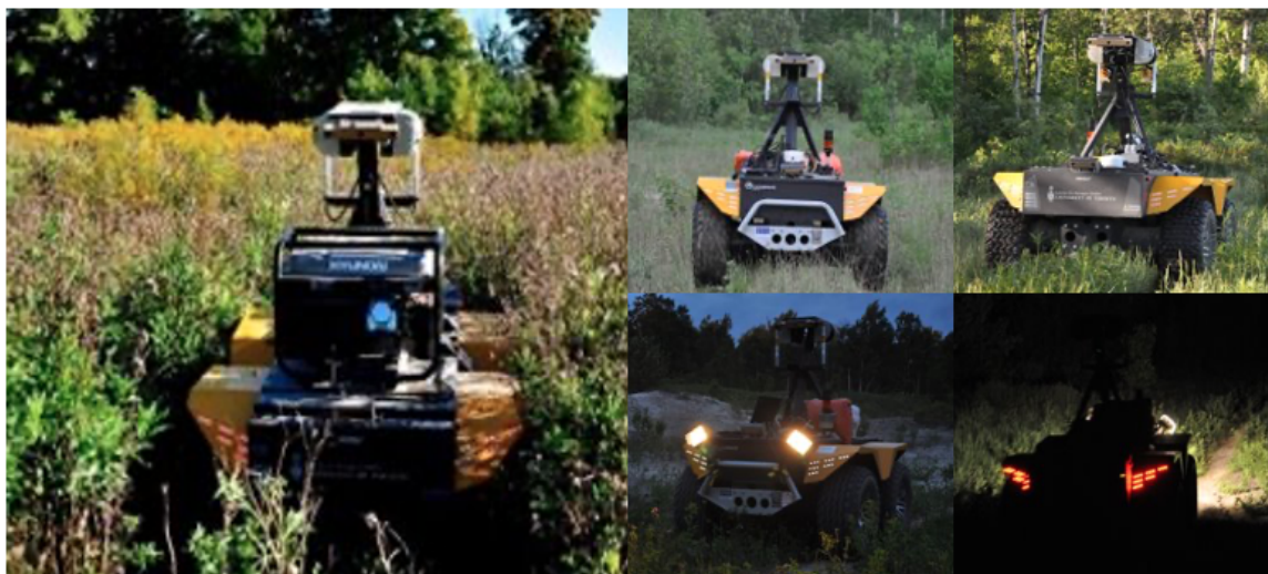
Figure 1.1: Grizzly ground robot autonomously repeats a taught path with learned features despite severe lighting changes.
