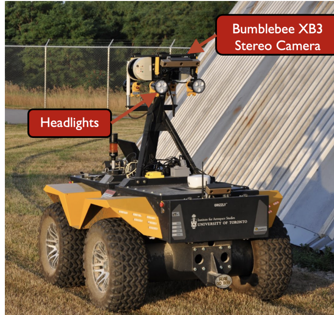
Figure 2.5: The Clearpath Grizzly Robot with a forward facing Bumblebee XB3 stereo camera and LED headlights.
