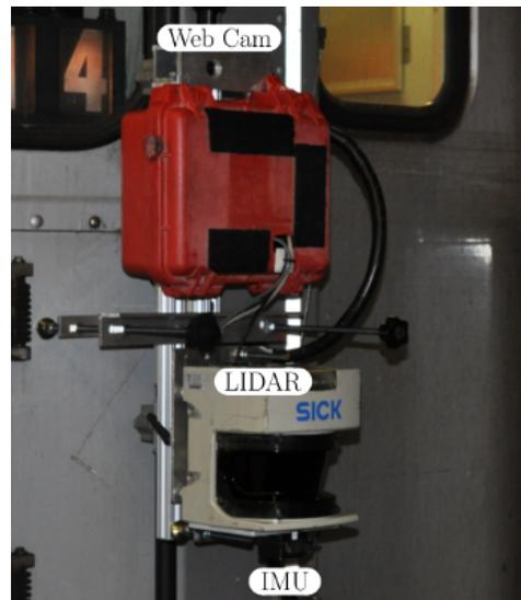
Figure 5.3: Experimental setup used to gather data in the subway tunnel. The sensor rig consisted of the SICK LMS291 lidar sensor, a microstrain IMU and a webcam.
