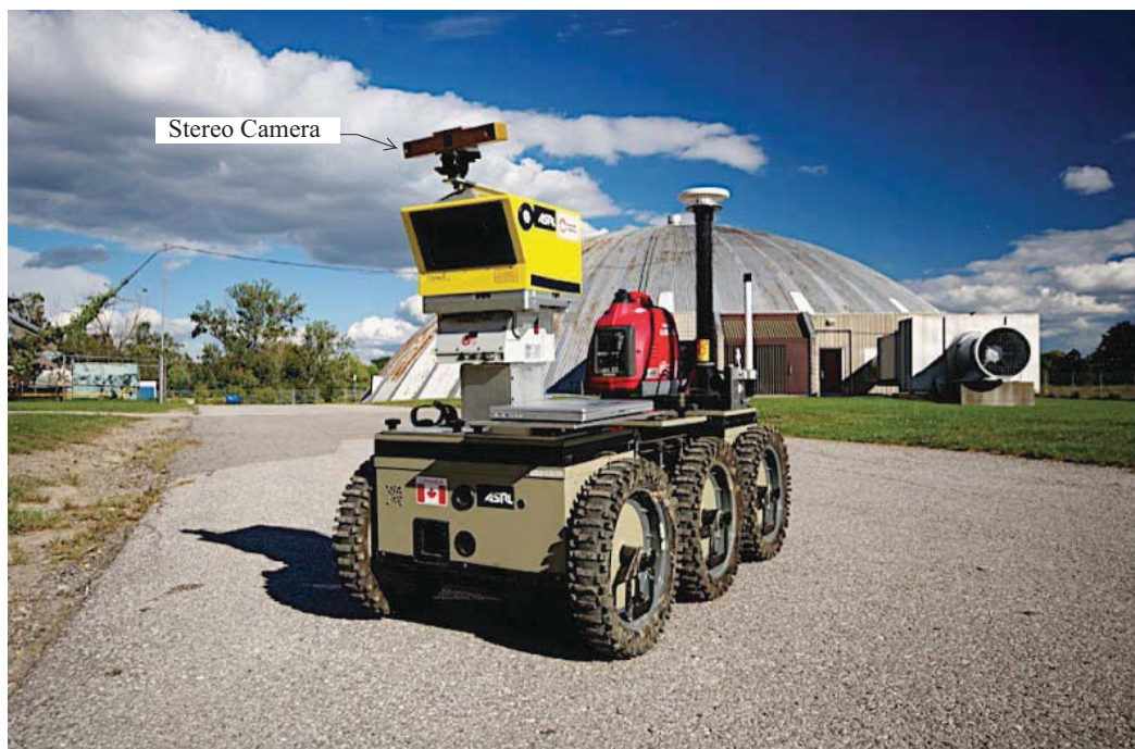
Figure 2.1: RO6 robot in ASRL facilities with an attached stereo camera. Photo credit: UTIAS/ASRL [2].
