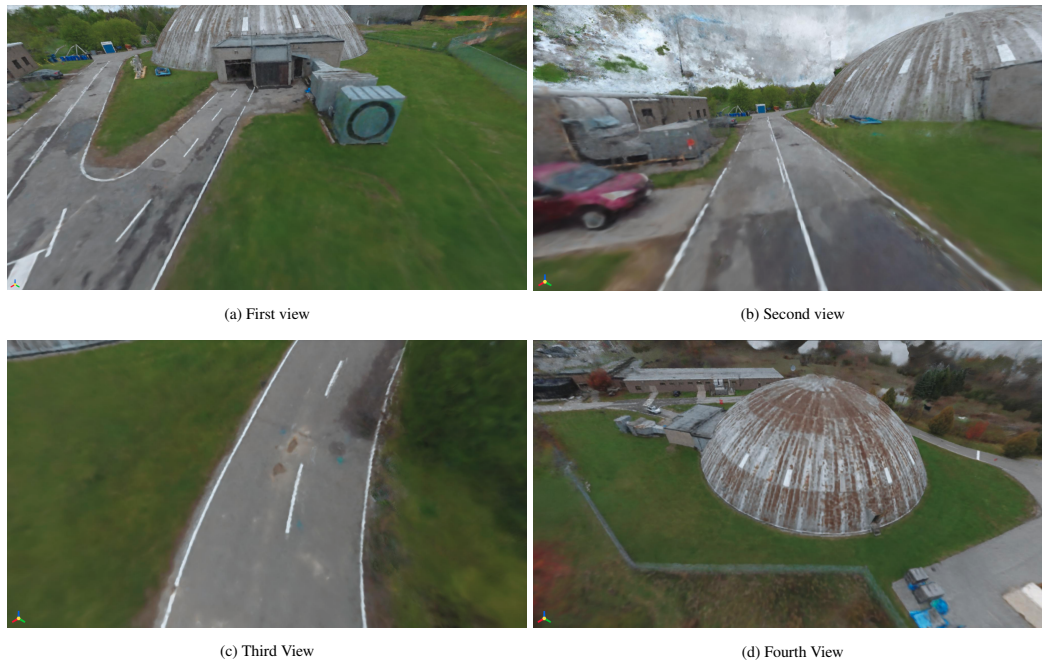
Figure 3.6: Several views of the NeRF volumetric rendering-based reconstruction of the UTIAS Mars Dome Loop dataset, created from aerial imagery taken by a drone and given to the software. Shown here is the volumetric rendering visualized in Nerfstudio. The detail captured in this dataset is consistent with all other datasets made by Nerfstudio with default parameters, where the spray paint marks, concrete cracks, grass texture, and many other details are visible.
