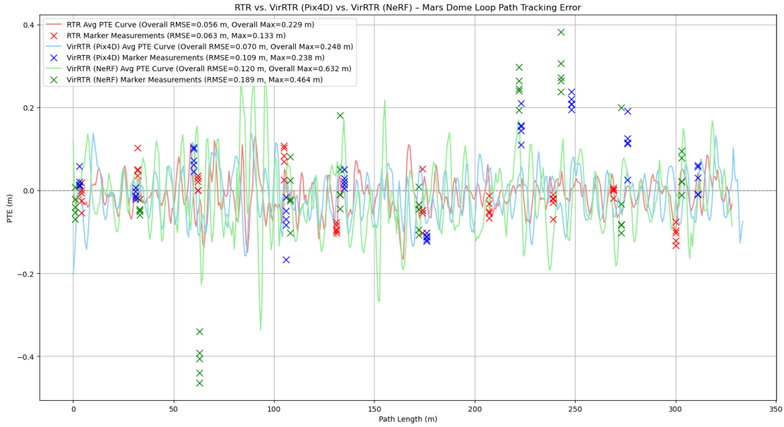
Figure 6.10: A comparison of Radar-based T&R algorithms on the Mars Dome Loop: RT&R (baseline), VirRT&R using Pix4D, and VirRT&R using NeRF (the overall worst configuration). Five measurements of the 10 markings are shown with the internally estimated PTE for the continuous route.
