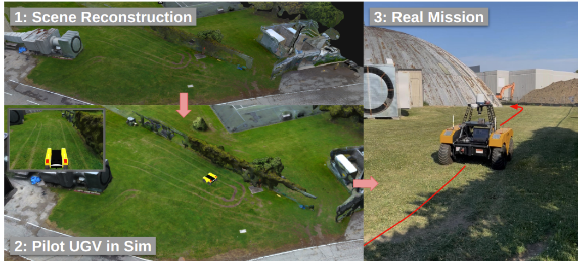
Figure 1.2: We present an architecture for navigating previously untraversed environments that uses 3D reconstruction tools to simulate the environment and create high-fidelity localization data from aerial imagery of the target environment. Shown here are the main steps of the framework, dubbed Virtual Teach and Repeat. The three steps are: 1. A scene reconstruction based on aerial imagery, a virtual driving simulation for virtual path definition, and the execution of an online mission with T&R.
