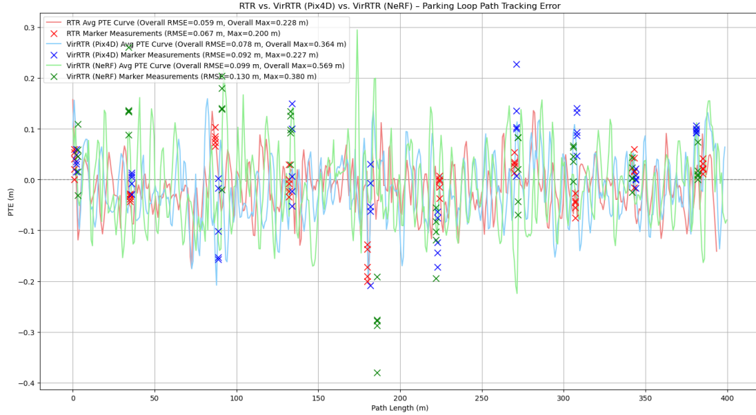
Figure 6.11: A comparison of Radar-based T&R algorithms on the Parking Dome Loop: RT&R (baseline), VirRT&R using Pix4D, and VirRT&R using NeRF (the overall worst configuration). Five measurements of the 10 markings are shown with the internally estimated PTE for the continuous route.
