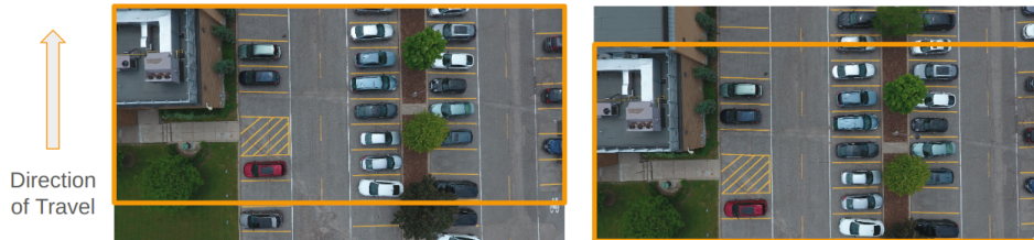
Figure 3.2: An example of approximately 80% overlap between images taken sequentially as a part of a dataset gathered for reconstruction with NeRF and Pix4D.
