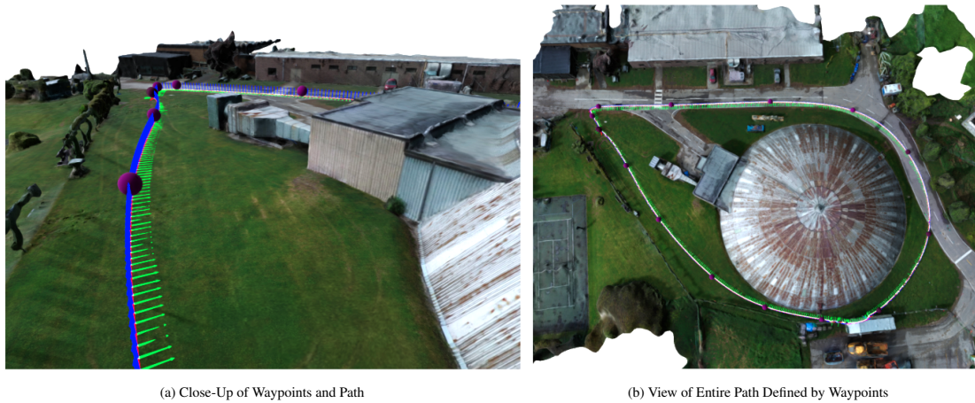
Figure 3.11: Views from the waypoint-based virtual path definition tool created for more efficient path generation, particularly for long paths. (a) Shows the interactive window panned closer to the spline fit between the purple waypoints used to define the path. (b) Shows the interactive window panned further to capture the whole path defined by the spline fit between the purple waypoints.
