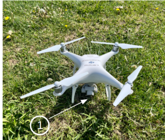
(b) Phantom Components: (1) Gimballed 1-inch 20 MP camera
