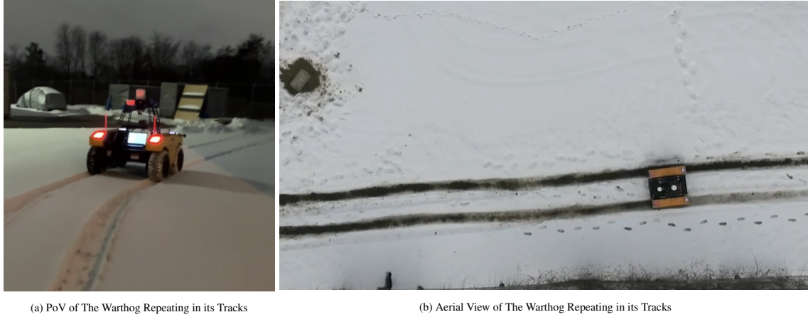
Figure 4.3: Visual evidence of low relative repeat deviations during real repeat missions using virtually generated teach maps on the Warthog. Relative repeat deviation can be qualitatively evaluated by observing no drift outside of tracks in the snow created by previous repeats.
