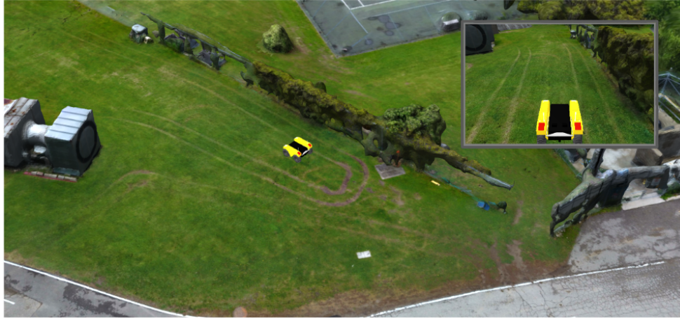
Figure 3.10: The URDF model of the Clearpath Warthog is being driven in the Gazebo pilot driving simulation that uses the triangular mesh virtually generated from the aerial scene reconstruction tools as the physical surface for traversal. The window in Gazebo shows the larger interactive view for panning around and the fixed PoV view of the robot placed at a 45^\circ angle above and behind the robot.
