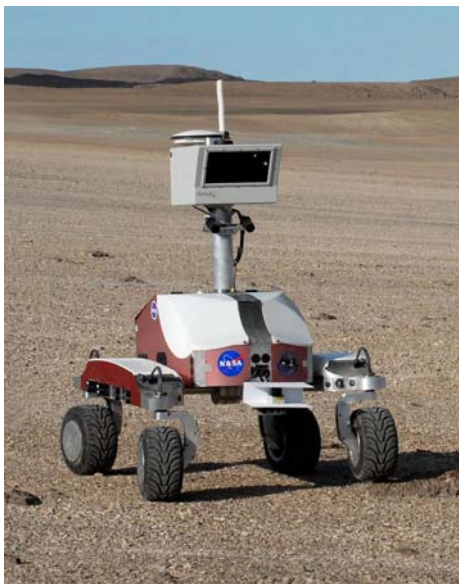
Fig. 12: NASA Ames K10 Rover Equipped with Optech ILRIS Lidar Credit: NASA
