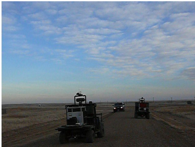
Figure 6.1: Oncoming vehicle may move into the path previously occupied by the leader vehicle.
