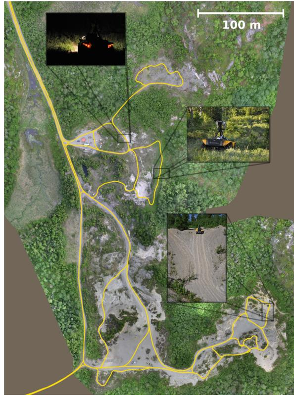
Figure 1.1: Orthomosaic imagery of the 5 km network of paths at the Ethier Sand and Gravel in Sudbury, Ontario, Canada. The map shows challenging environmental uncertainties for robust route planning: lighting change, shifting sand with little visual texture, and dense vegetation with changing appearance.
