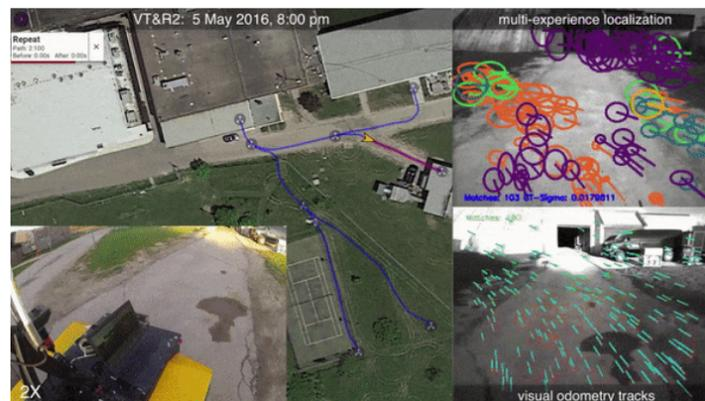
Figure 2.5: Live demonstration of the VT&R algorithm. The left panel shows the privileged (teach) paths layered on top of the satellite map. The bottom-left corner shows the image of the robot. The bottom-right corner shows the features extracted from the live image as well as the visual odometry track. The top-right corner shows the matched features from the live image to previous experiences over the path, with different colors indicating feature matches from different experiences.
