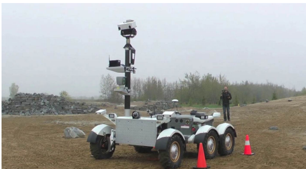
Figure 14: Successful VT&R traverse spanning the length of the CSA AT, returning to the starting point (marked by orange cones).
