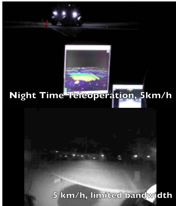
Figure 9: Night time tele-operation test at 5 km/h in the MDA parking lot. Top: External view of rover and live 3D point cloud and drive camera displays. (Note that operator could not directly observe the rover during the actual test.) Bottom: Drive camera view compressed to meet the lunar bandwidth constraint.
