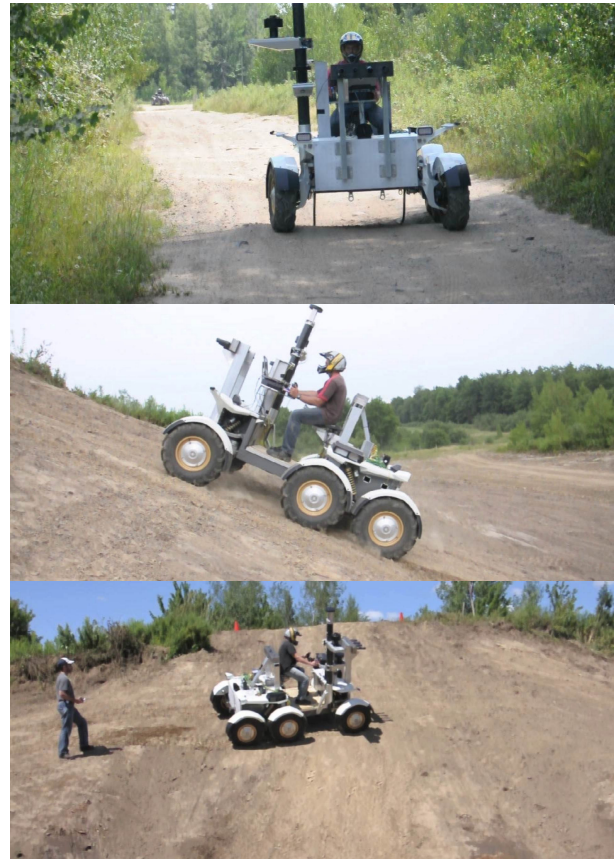
Figure 8: Core vehicle tests at BRP's ATV proving grounds (top), including 25° slope climbing (middle) and cross hill traverse (bottom).
