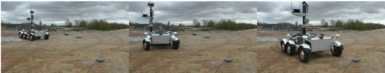
Figure 13: Hercules performing an autonomous precision drive to place the rock within the workspace of the rover.
