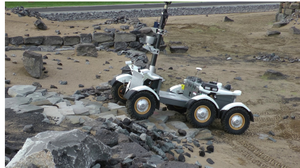
Figure 10: Climbing the stairs at CSA AT during tele-operation test with 700 kbit/s bandwidth limit and 3 second delay.
