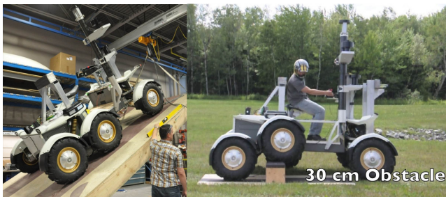
Figure 7: Some initial tests at CTA-BRP: static slope stability (left) and 30 cm obstacle crossing (right).
