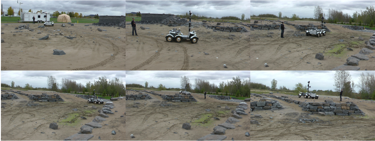
Figure 12: Hercules performing a fully autonomous drive in the CSA AT. Still frames show the rover successfully executing the traverse shown in Figure 11.
