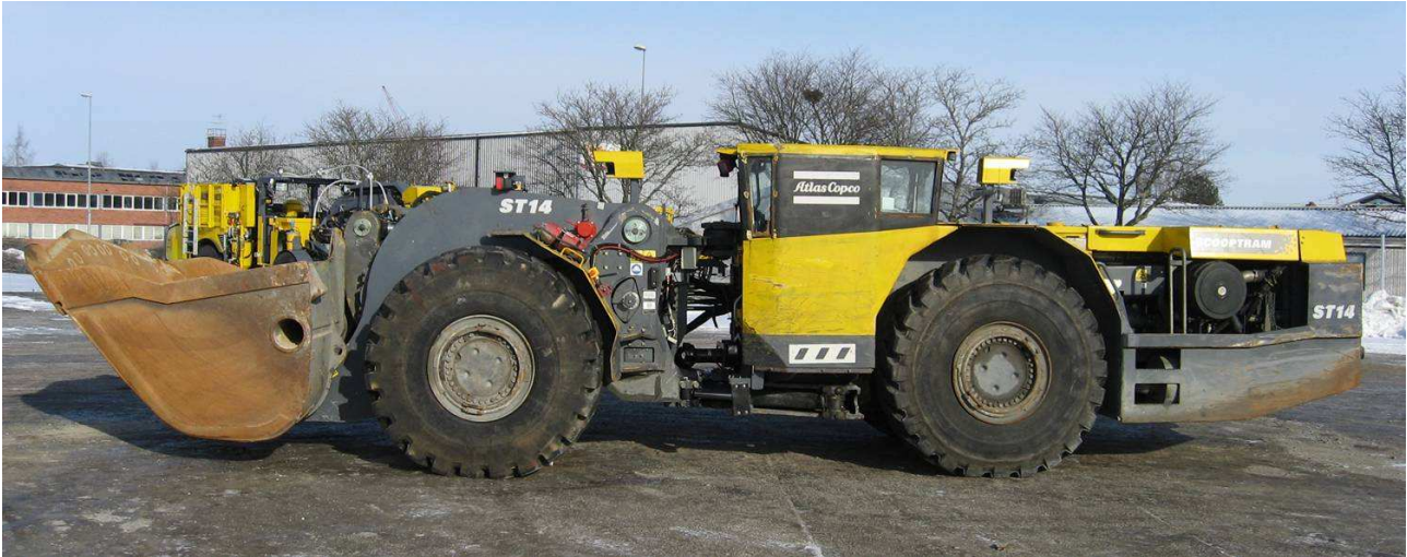
Figure 4 Atlas Copco ST14 Scooptram test vehicle, the sensor layout is the same as for the ST1010C. The IMU is mounted in the housing of the front laser scanner.
