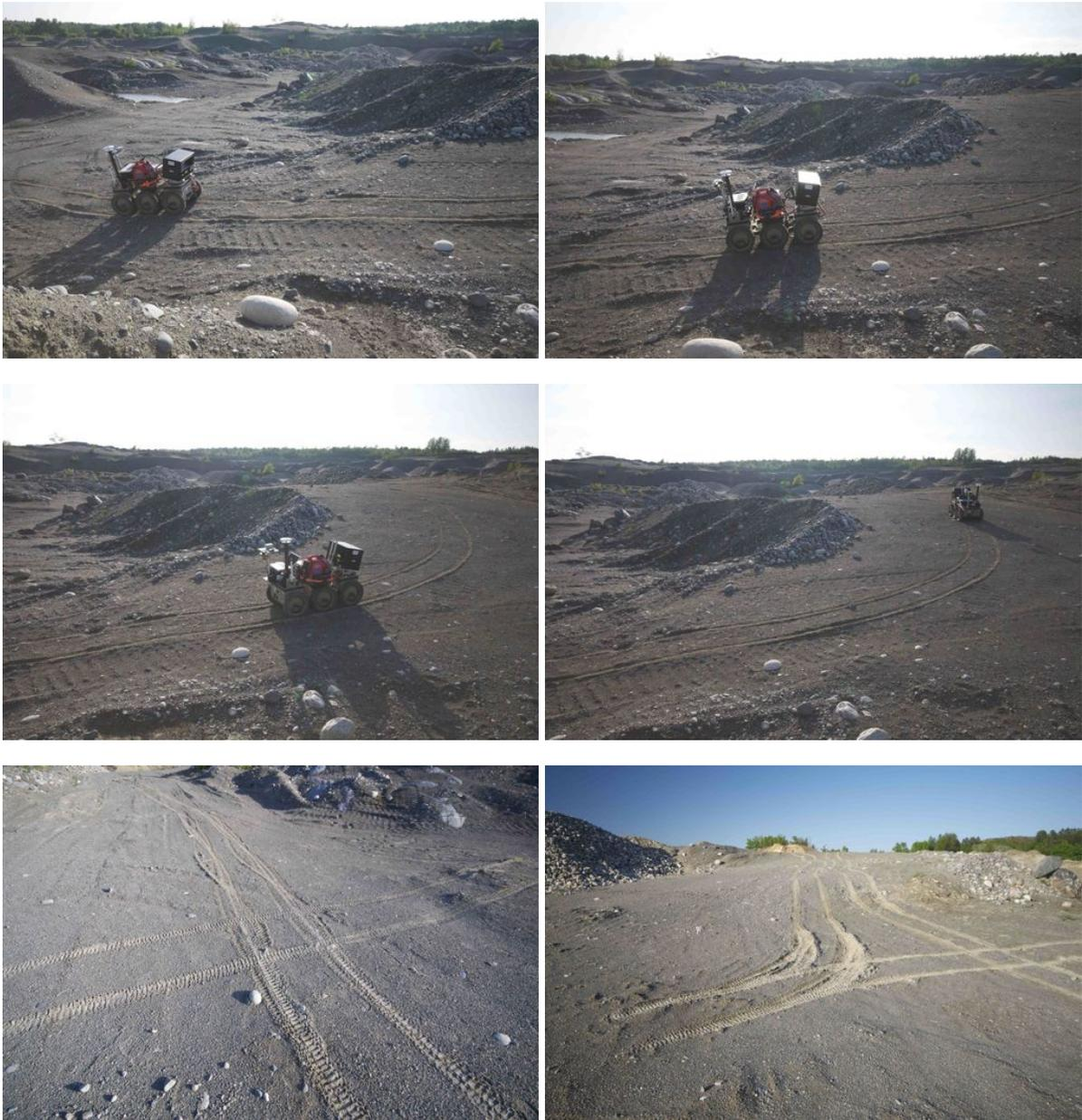
Figure 8.7: Images of an autonomous repeat, where the robot can be seen driving in its own tracks off in the distance. The bottom row shows some of the tracks that were repeatedly traversed over all 10 runs.
