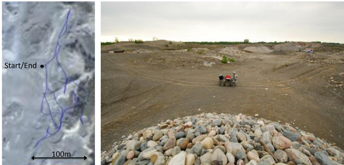
Figure 7.1: Left: a GPS track of the 1154m taught route in the Etheir Sand and Gravel pit in Sudbury, which proved to be an effective analogue environment due to its lack of vegetation and 3D terrain. Right: an image of the ROC6 field robot during an autonomous repeat traverse.
