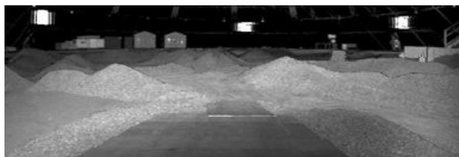
(d) Processed Autosys intensity image with a linear range correction. Note that distant features are more visible.
