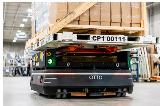
(b) Autonomous warehouse robot. Photo credit: OTTO Motors (2020).
