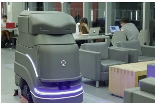
(a) Autonomous floor cleaning robot. Photo credit: Avidbots (2020).
