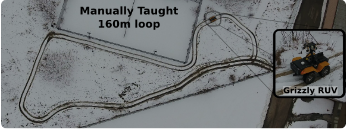
Figure 5.11: A Grizzly RUV deployed with the VT&R 2.0 system navigating a small 160m loop at the University of Toronto Institute for Aerospace Studies (UTIAS) during the 2017 multi-season field test. This field test demonstrates the VT&R 2.0 system’s ability to autonomously operate over long time periods. Over the course of four months the robot autonomously repeated this loop 163 times experiencing appearance change as extreme as snow, freezing rain, and vegetation growth.
