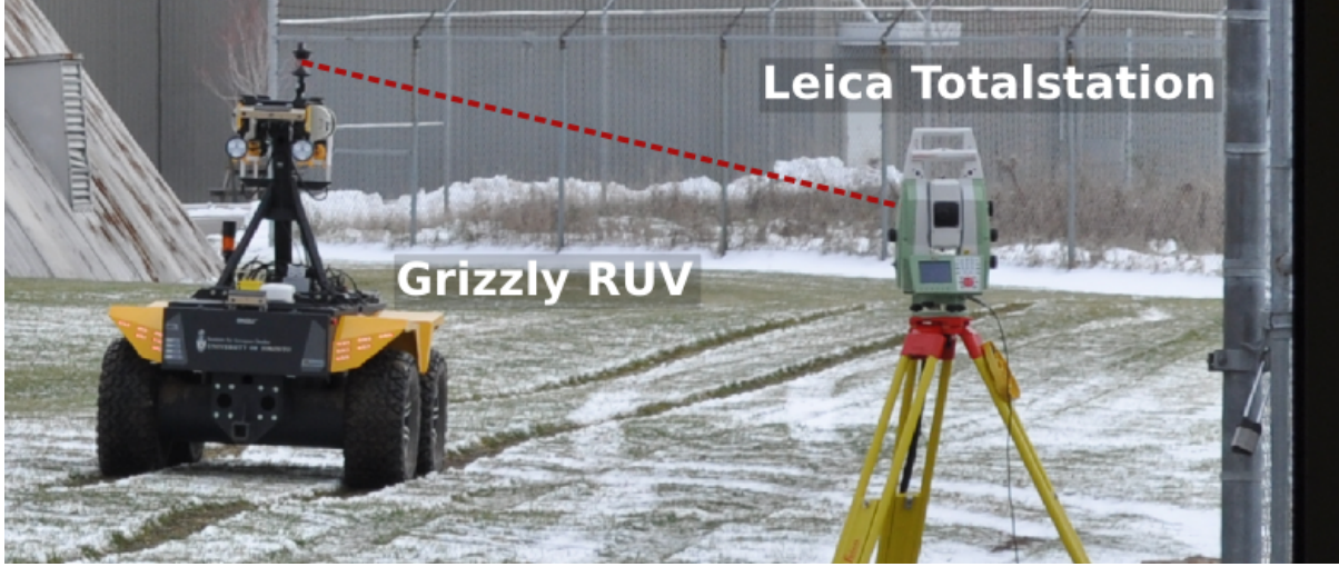
Figure 4.9: Setup for the photocopy-of-a-photocopy experiment. This experiment was conducted to help quantify the spatial drift incurred in MEL algorithm. Translational ground truth was collected with a Leica Totalstation tracking a prism on a Clearpath Grizzly RUV.
