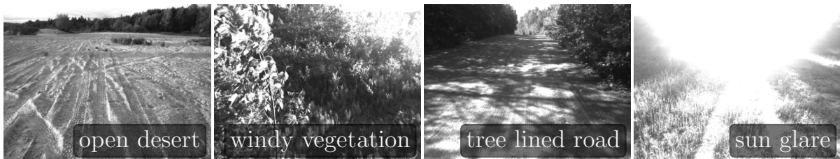
Figure 5.30: Example images of areas that remain difficult for vision-based navigation. from left to right: i) open desert areas with heavy vehicle traffic, ii) lush vegetation during high winds, iii) tree-lined corridors with strong shadows, and iv) sun glare.
