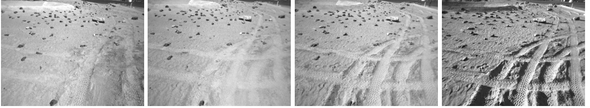
(b) Impact of the sun and robot in desert environments. Small textures such as rocks and wavy sand cast shadows and vehicles driving in sand significantly alter the terrain in a short amount of time. This sequence shows the same scene at different times of day, namely, at 11:03, 13:15, 15:12, 17:49
