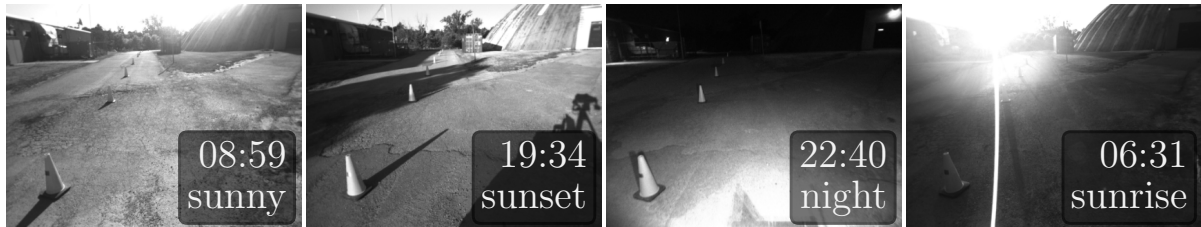
Figure 5.10: Examples of the appearance change observed during the 30-hour UTIAS In the Dark field test. This short field test demonstrates the VT&R 2.0 system's ability to handle many experiences of a single scene in one map (40+) as well as operate continuously over a 24-hour period with on-board headlights illuminating the scene at night.
