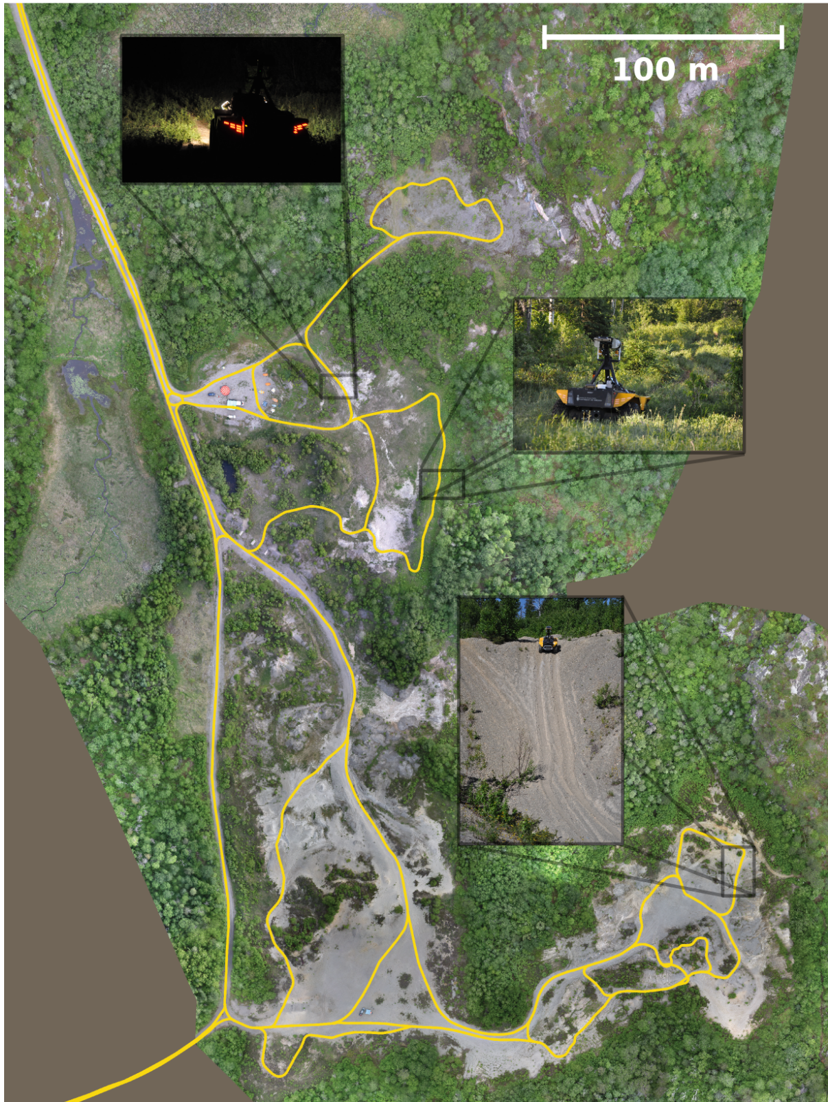
Figure 5.7: Orthomosaic imagery of the 5 km network of paths at the Ethier Sand and Gravel in Sudbury, ON. This network was taught during a 10 day field trial to experimentally validate the VT&R 2.0 system’s ability to perform long-range, long-term vision-based autonomous path following in difficult environments, highlighted in the image. Over the course of the field test, the robot autonomously traversed 140 km with an autonomy rate of 99.59% of distance traveled.
