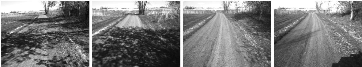
Figure 2.5: Example of daily appearance change due to lighting on a sunny day. This sequence shows the same scene at different times of day, namely, 10:58, 13:10, 15:17, and 17:44. On sunny days such as this, the operational window of the VT&R 1.0 system is limited to only a few hours.
