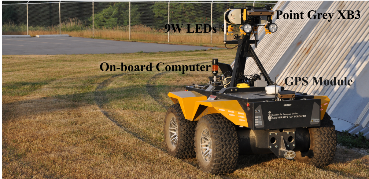
Figure 5.6: Clearpath Grizzly RUV and its sensor configuration. The robot is equipped with a forward- and rear-facing PGR Bumblebee XB3 cameras, a GPS receiver, and four 9W LED headlights for night-time operation. The robot contains a ROS enabled embedded computer that controls its motors and safety monitors.
