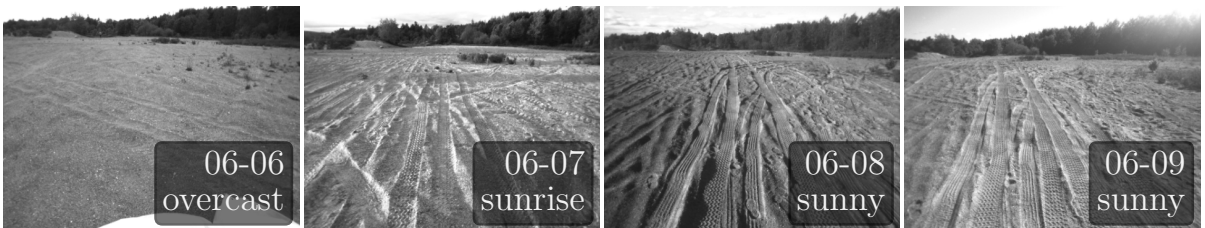
Figure 5.27: Appearance change in an open desert area of the 5km network of paths. In this section of the network, appearance change manifested from external lighting, shifting sand, and vehicle tracks. The lack of stable features apart from the treeline on the horizon make this environment especially difficult for vision-based navigation.
