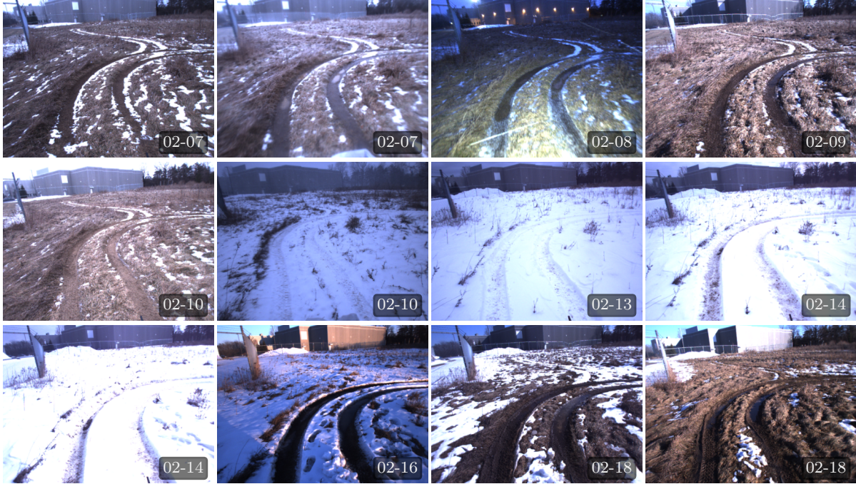
Figure 4.15: Rapid appearance change examples in the UTIAS multi-season field test. Each row shows the rapid appearance change over the course of a few days. top row : experiences 20-30, the appearance of the scene changes from light snow fall to freezing rain to snow melt. middle row : experiences 38-51, the appearance of the scene changes from little snow to light snow to heavy snow in four days. bottom row : experiences 58-68, the appearance of the scene changes from heavy snow to snow melt in four days.
