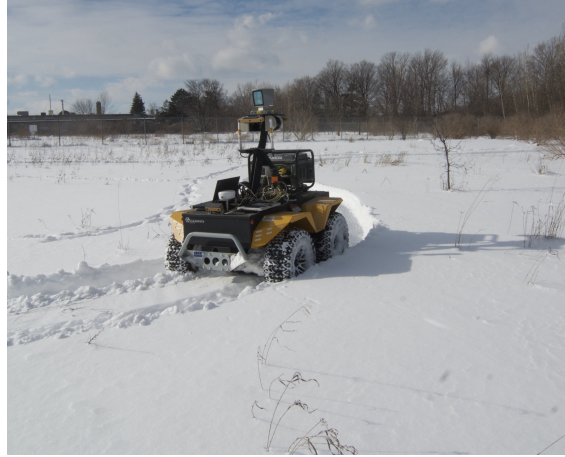
Figure 3.24: Photograph from an attempted autonomous traversal in the deep snow. A lack of visual keypoints in the foreground resulted in poor localization and VO estimates.
