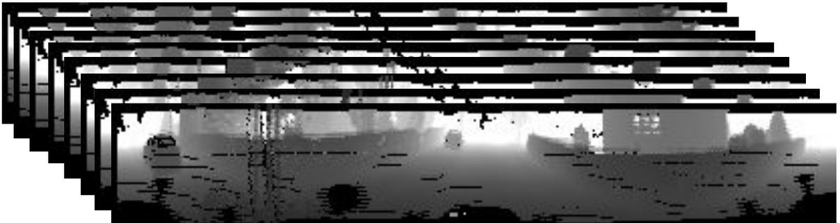
Figure 4.8: A  $360 \times 64 \times 8$  tensor range image used as input to the CNN model.
