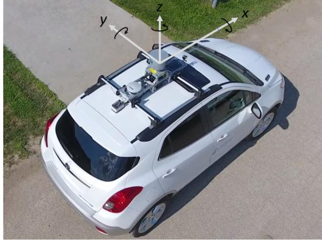
Figure 4.1: The coordinate system used by our odometry algorithm. Roll, pitch, and yaw are rotations about the  $x$ ,  $y$ , and  $z$  axes, respectively.
