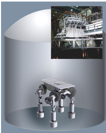
Fig. 9, Artist's rendition of the lunar rover chassis in a test fixture in a thermal vacuum chamber to emulate the lunar environment for testing.
