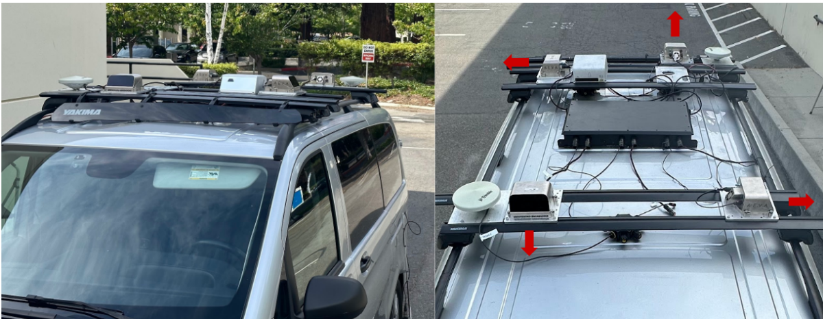
Figure 5.6: Images of the data collection platform used for the Aeva HQ dataset. The platform is equipped with four Aeries II FMCW lidar sensors and a Applanix POS LV for providing groundtruth. Each sensor is facing in a different direction (i.e., forward, left, right, and back), which is indicated by the red arrows in the right image.
