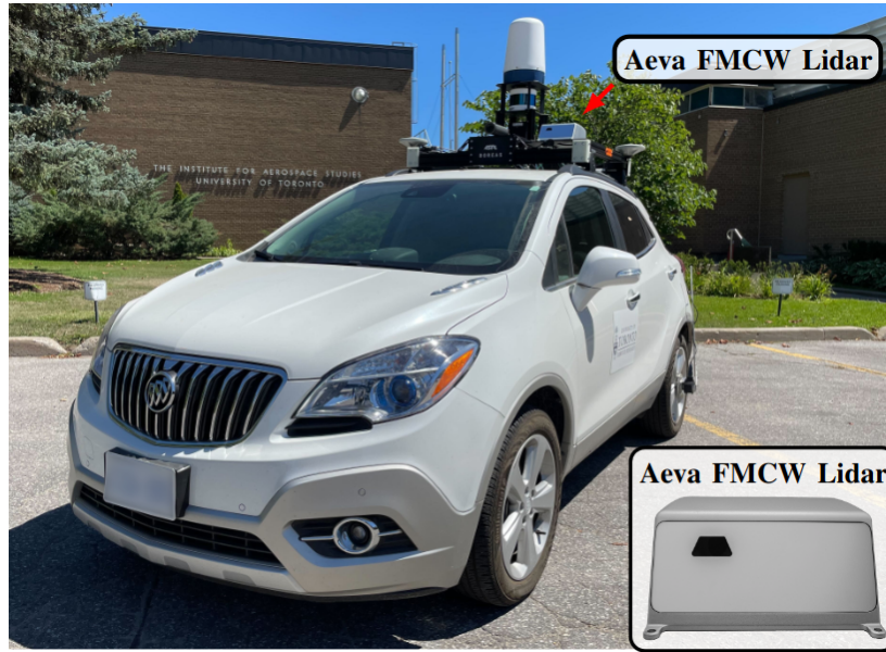
Figure 5.4: Our platform, Boreas , was previously used to collect the Boreas Multi-Season dataset (Burnett et al., 2023) and additionally equipped with an Aeva Aeries I FMCW Lidar for use in this work.
