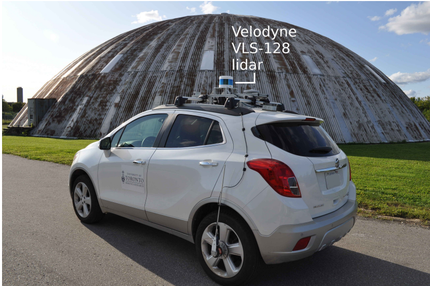
Figure 4.1: The data collection vehicle used for our lidar localization experiments. The vehicle is equipped with a Velodyne VLS-128 lidar and an Applanix POS LV for the groundtruth trajectory.
